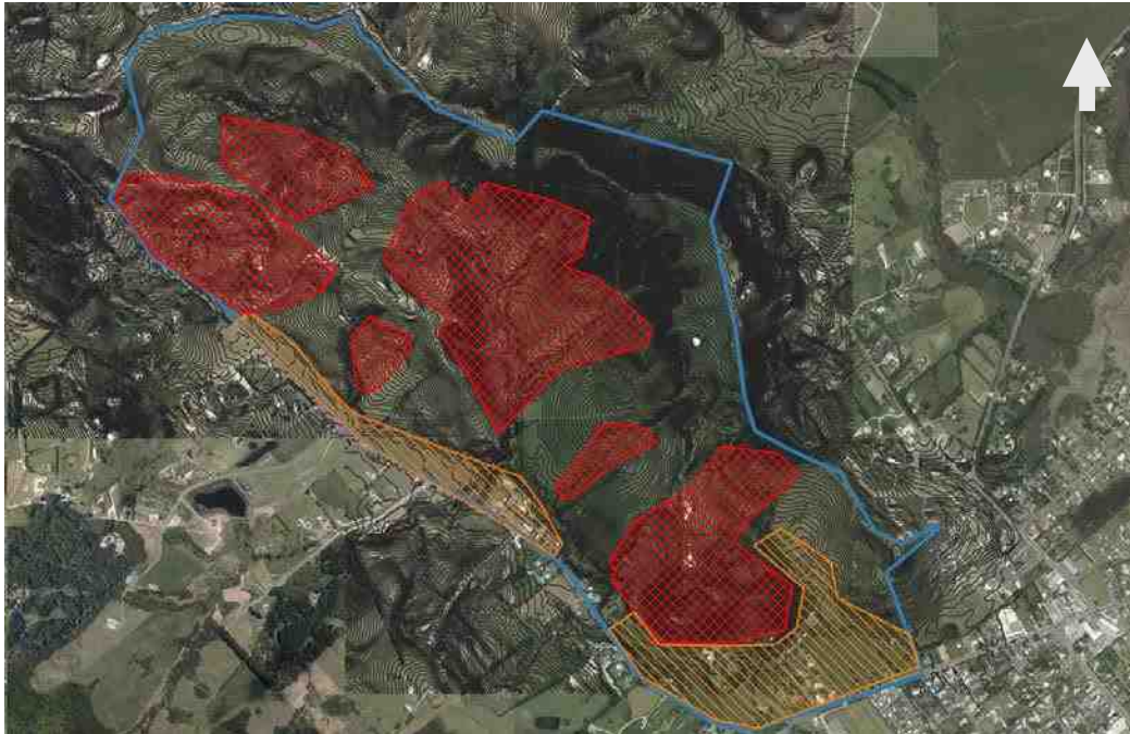
Figure C – GIS model of the subject site with 1.0m contours. (Source: QGIS and Northland LiDAR data). Red hatching indicates areas potentially prone to high slope instability hazard, and orange low-lying land susceptible to moderate settlement/liquefaction (subsidence) hazards.
